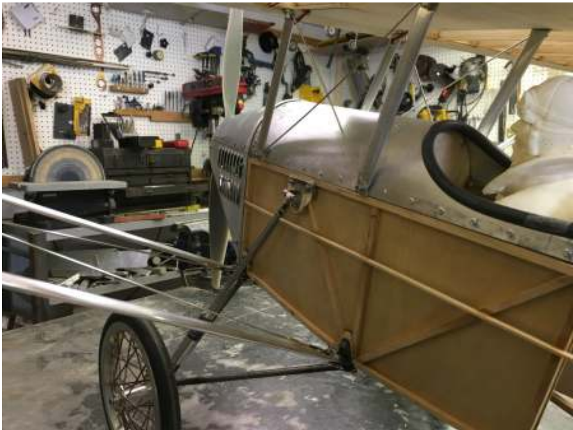
A Don Davis creation. From plans a 1/4 scale Pietenpol Sky Scout. Everything you see was fabricated by Don. Including the wheels. Amazing work.
